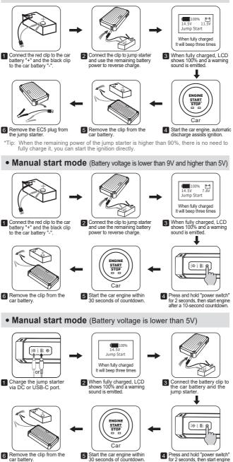
\*Tips: 1. In manual start mode, the remaining power of the jump starter must be higher than 90%; 2. If the car battery is too low in power or severely aged, or the voltage is extremely low, a large-displacement car may not be able to start; you can repeat the operation and try to start the ignition multiple times.
